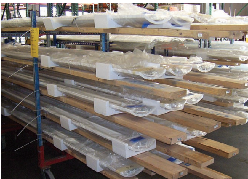
Photo 1. Prefabricated “ready assembly” packages are assembled in the SASCO Electric prefabrication warehouse. This ensures that excess packaging never makes it to the jobsite.
